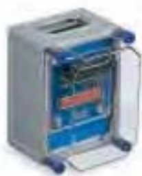
SAFE SERIES Fuse-holder unit in watertight modular container in insulating material with internal cap for protective insulation 500V IP65
