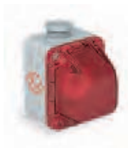
TAIS-MIGNON-Ex SERIES ATEX signal lamps in watertight wall-mounted enclosure thermosetting (GRP) material with E14 lampholder IP65
