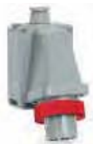
CEE SERIES Watertight wall-mounted 90° angled fixed appliance inlets In = 63A, high performance and low voltage, enclosure in thermosetting (GRP) material IP65
