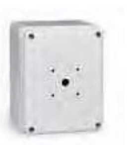
CAM-ST series Wall-mounted enclosure with provision for front panel control of a rear panel device screw fixing IP65
