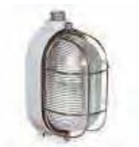
RINO SERIES Grey watertight oval lighting fixtures in aluminium alloy RAL 7035, tropicalized steel wire protective cage, and glass diffuser 250V - IP65
