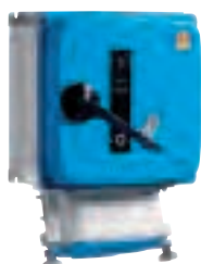
TUNNEL54 SERIES Interlocked socket-outlets for tunnel fans IP66 > IK10 400°C for 120'
